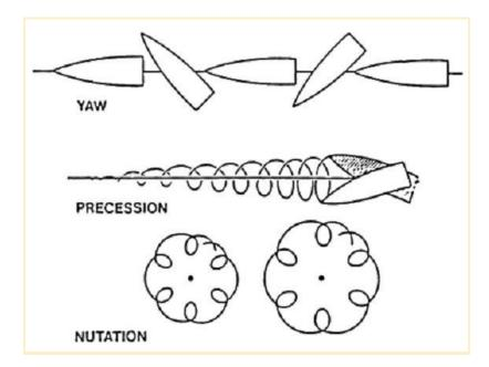
Yaw refers to the rotation of the nose of the bullet away from the line of flight. Precession refers to rotation of the bullet around the center of mass. Nutation refers to small circular movement at the bullet tip. Yaw and precession decrease as the distance of the bullet from the barrel increases.
