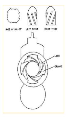
Bullets do not typically follow a straight line to the target. Rotational forces are in effect that keep the bullet off a straight axis of flight. These rotational effects are diagrammed below:
